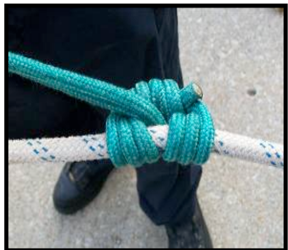
Figure 2.1 – “FLP” or Bridged Prusik Loop
