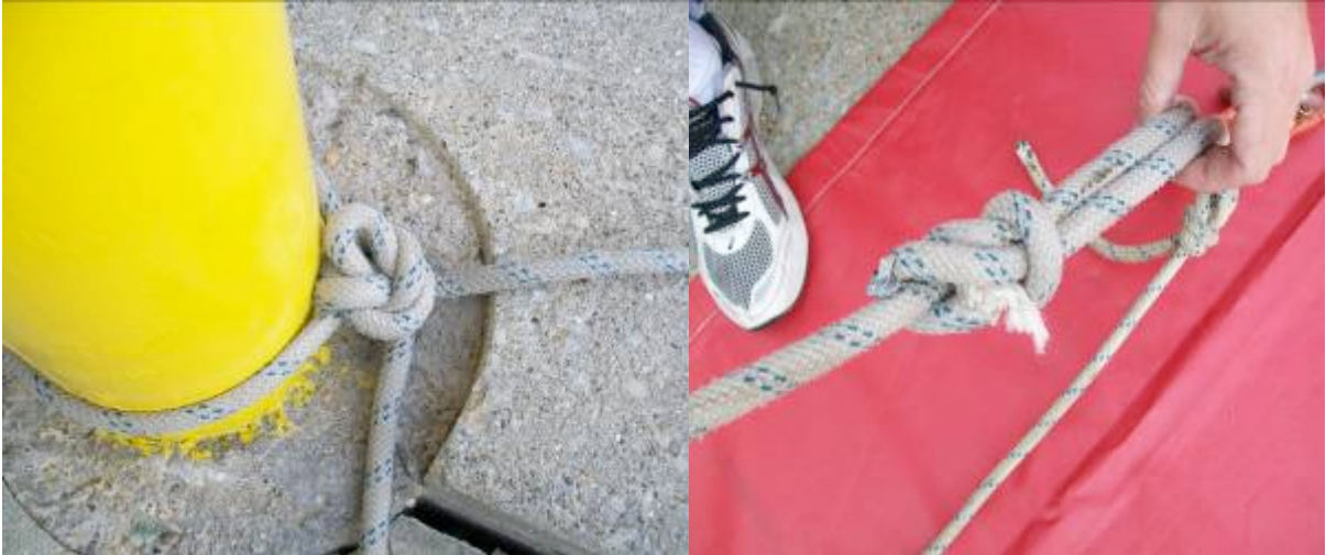
Figure 8.4 - Double Beckett after several load tests, Figure 8.5 - Failed Figure 8 on bight
