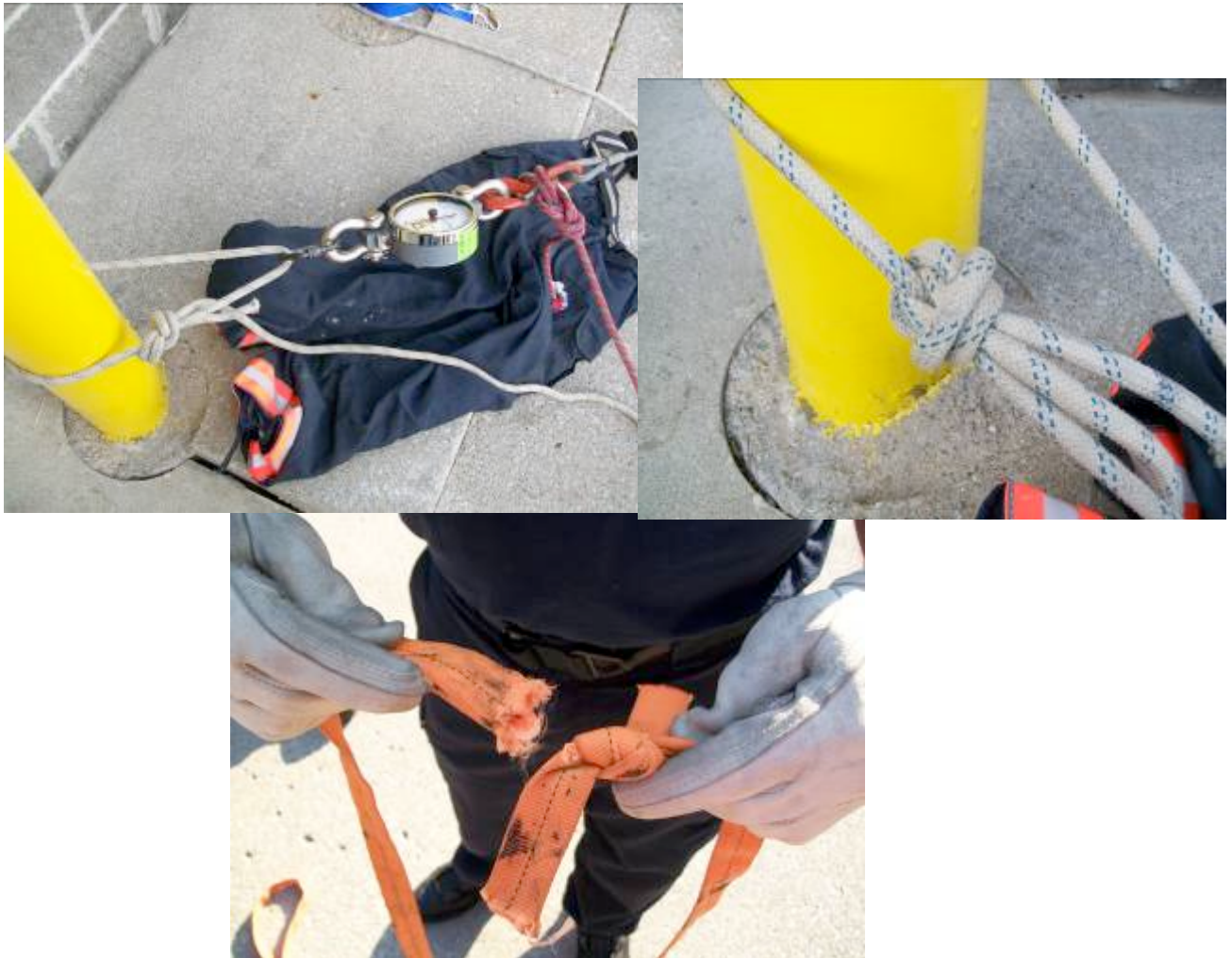
Figure 8.1, 8.2 – Double Beckett, 8.3 – Failed webbing at water knot
