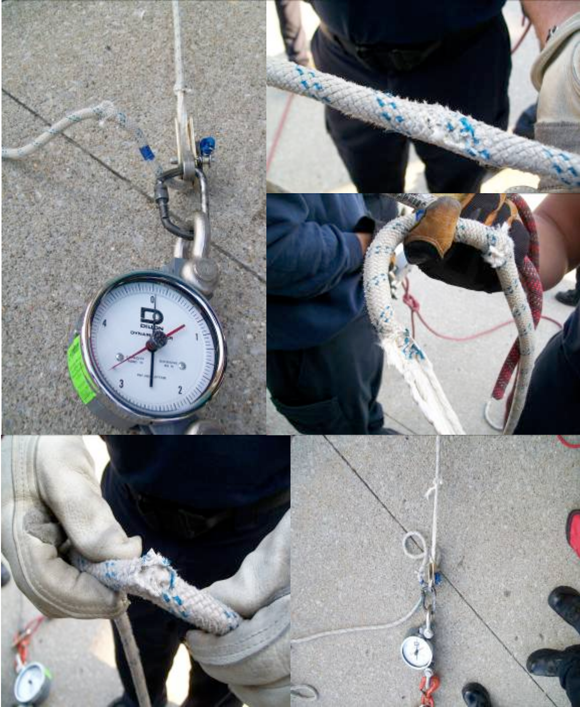
Figure 3a.1 – Montage of Gibbs Ascender failures
