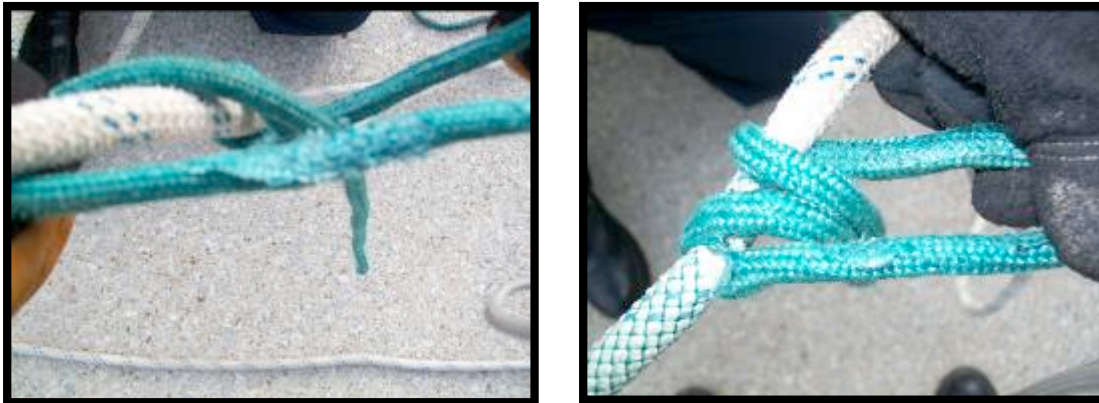
Figure 2.2, 2.3 – Old prusik loop failure with melting and residual on haul line
